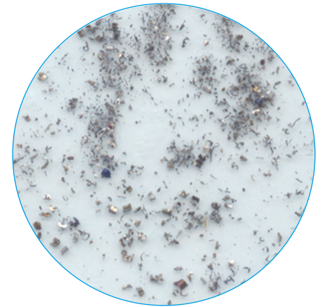
Metallic particles from a hydraulic pipe cut on both ends
